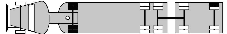
All tires on the drive axle and one tire on either side of the last axle of the last trailer.
