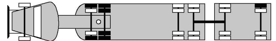
Only on six or more axle combinations when posted "ALL VEHICLES CHAINS REQUIRED" one additional tire on each side of the drive axle shall be chained.
